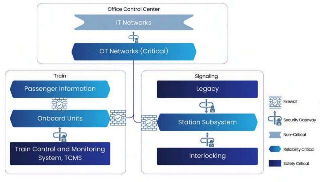
Security zones, as defined by IEC 62443, group logical or physical assets that share common security requirements. These zones can be hierarchical and include subzones, which help segregate equipment based on different communication needs. Categorizing networks into three levels of criticality—safety, reliability, and efficiency—simplifies network security procedures and protocols.
