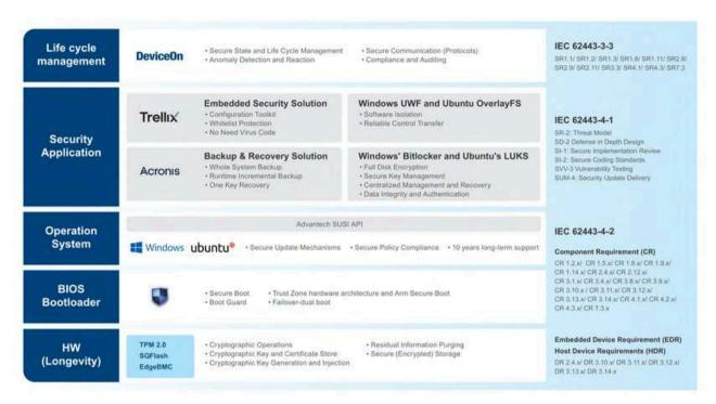
Advantech provides robust security capabilities such as secure boot, access control, secure communication, security monitoring, firmware updates, and physical security measures. These features align with the foundational requirements outlined in IEC 62443-4-2, empowering OEMs to construct secure and resilient industrial control systems.
