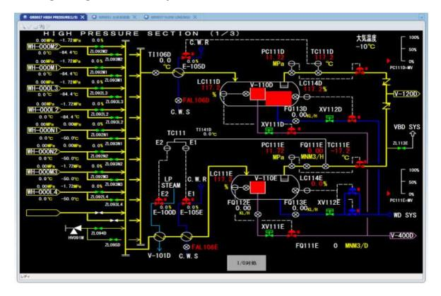
On the process graphics, pumps are red because they are not running, and green because they are running. On the electrical distribution graphic, motors are red because they are live (running) and green because they are not live (stopped). The separation column temperature half way up the column is red because it is in high alarm.
