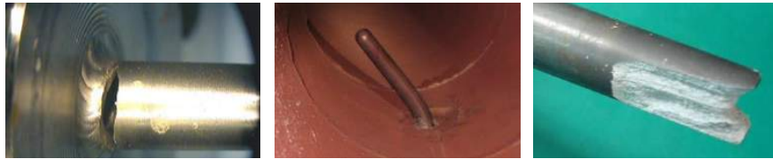
Figure 2. Examples of Thermowell Failure
