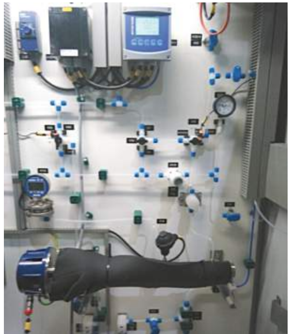
GPro 500 with insulation and the extractive system
