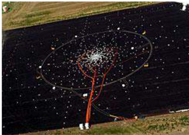
Figure 19. By using a PXI architecture configured for mass synchronization across multiple chassis, Boeing synchronized more than 600 ground-based microphones for data acquisition while reducing cabling and cost per channel.
