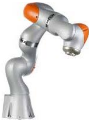
Kuka’s “LBR iiwa” Lightweight Robot with Integrated Forces Sensor in Each Joint
