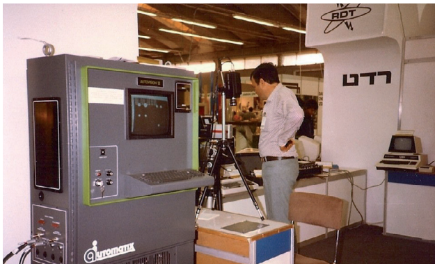
Early Automatix Inc machine vision system at a trade show in 1983. The camera on a tripod is pointing down at a light table to produce a backlit image, which is then processed in the monolithic controller, probably employing a 68000 microprocessor.
