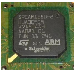
M580 ePAC's ARM Microprocessor
